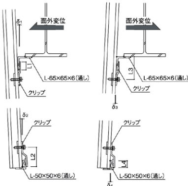
$$\begin{aligned}\delta_1 &= L1 \times 1/100 \\ \delta_1 &= 35 \times 1/100 = 0.35\text{mm} \\ \delta_2 &= L2 \times 1/100 \\ \delta_2 &= 95 \times 1/100 = 0.95\text{mm} \\ \delta_3 &= L3 \times 1/100 \\ \delta_3 &= (85 + 30) \times 1/100 = 1.15\text{mm} \\ \delta_4 &= L4 \times 1/100 \\ \delta_4 &= 32.5 \times 1/100 = 0.325\text{mm}\end{aligned}$$
