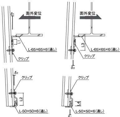
$$\begin{aligned}\delta_1 &= L_1 \times 1/100 \\ \delta_1 &= 35 \times 1/100 = 0.35\text{mm} \\ \delta_2 &= L_2 \times 1/100 \\ \delta_2 &= 95 \times 1/100 = 0.95\text{mm} \\ \delta_3 &= L_3 \times 1/100 \\ \delta_3 &= (85+30) \times 1/100 = 1.15\text{mm} \\ \delta_4 &= L_4 \times 1/100 \\ \delta_4 &= 32.5 \times 1/100 = 0.325\text{mm}\end{aligned}$$
